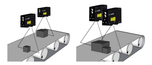
If there is an overlap between the FoVs, you will need to shift the exposure times so that the laser from one Matrox AltiZ unit does not interfere with that of the other.
