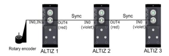
In the case of an overlap between the FoVs, acquisition for the following AltiZ in the chain is triggered by the falling edge of the **Exposure Active** signal from the previous AltiZ in the chain. In the daisy chain configuration, the exposure is limited to half of the Acquisition Line Period, minus the ON to OFF response time
