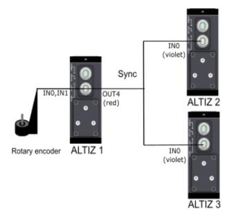
In our example, we connected AUX\_OUT4 of ALTIZ 1 to AUX\_IN0 of ALTIZ 2 and 3. Other input and output pins can be used, as long as they are free.
